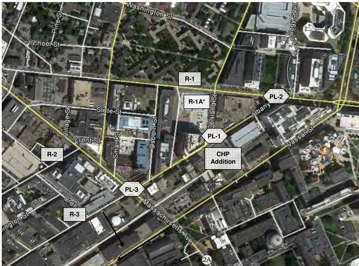
Figure 3. Aerial Photograph Showing Planned Location for MIT CHP Addition and Distances to Property Line (PL) and Residential (R) Locations for August 2014 Ambient Sound Survey and Analysis.
